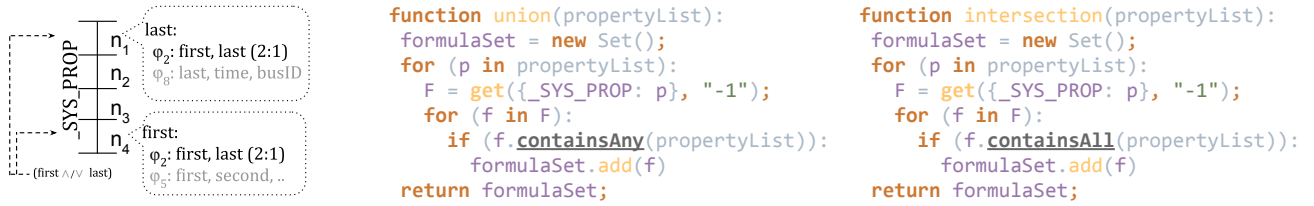
Figure 3: Use of inverted formulas and queries on structure. Union returns \phi_2 , \phi_8 , and \phi_5 ; intersection returns \phi_2 .
