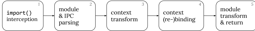
Figure 5.4: Transformation pipeline. Module loading is augmented with several stages that transform the module and its context before returning its value to the importing code. Stages (1), (3), and (5) manipulate in-memory objects; stages (2) and (4) operate on source code (Cf. §5.5).
